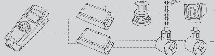
2 windlasses (up/down) plus deck wash and deck light for each windlass
