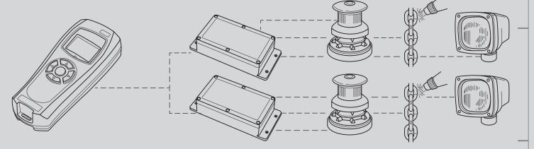
2 windlasses (up/down) plus a bow thruster (port/starboard) and a stern thruster(port/starboard) Note: Both thrusters can be operated simultaneously
