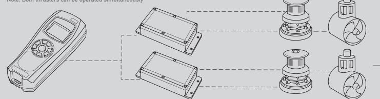
EXTRA CONSOLES: A system can be operated by up to 3 consoles.
