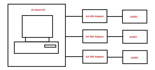
Note: The AA-485 adapter should be connected either direct to the PC USB port or through a powered USB hub.
